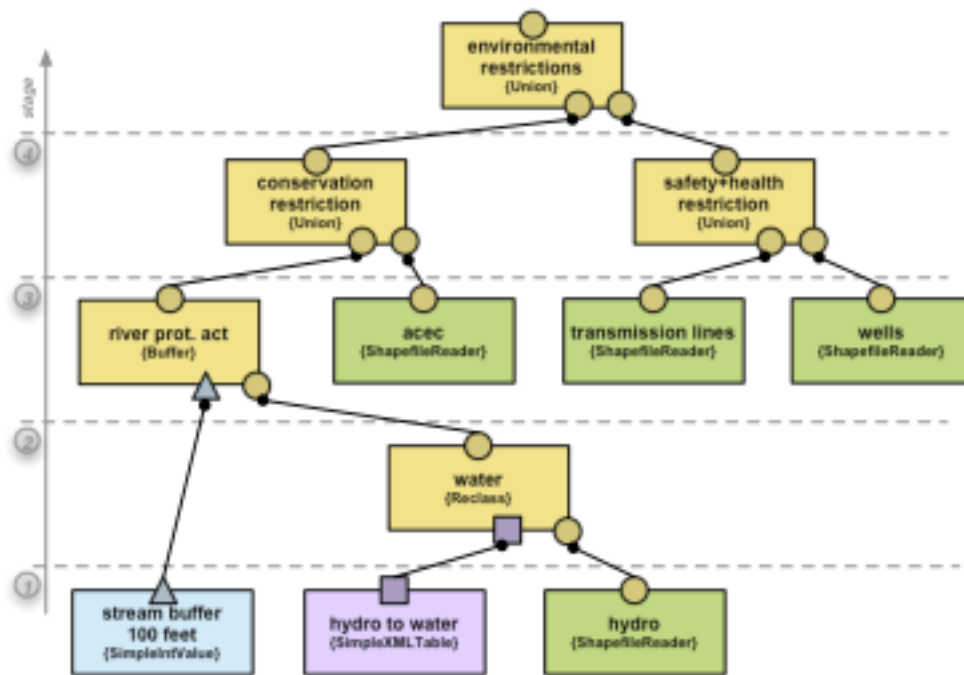
Figure 6-6: PAMML model of land that is exempt from development for environmental reasons
